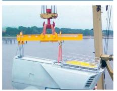
Lifting / manipulating beams and Up-ending tools
